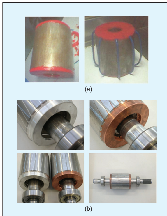
FIGURE 4 – (a) Copper cage prototype preparation and (b) aluminum and copper rotors.
