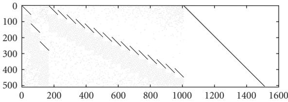
FIGURE 4: Parity-check matrix of a (1512, 1008) code.
