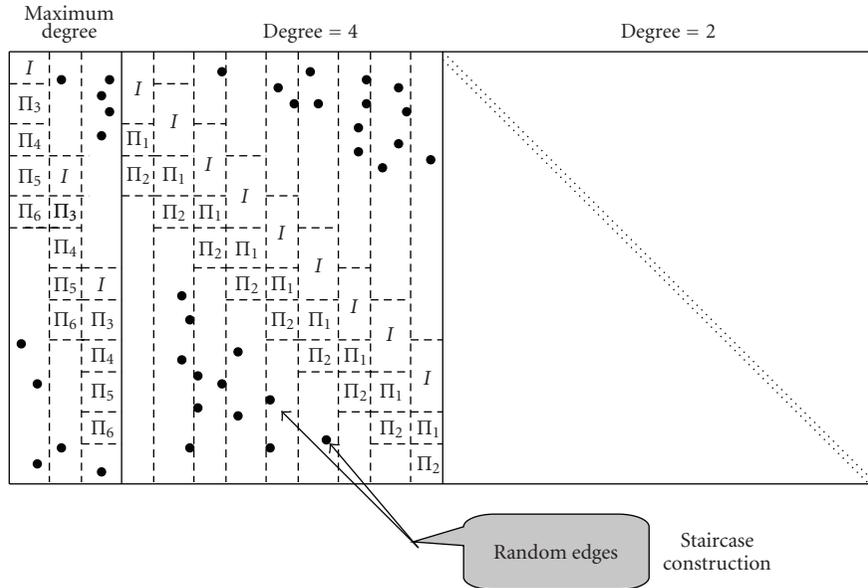
FIGURE 1: Parity-check matrix structure for code rate 1/2.
