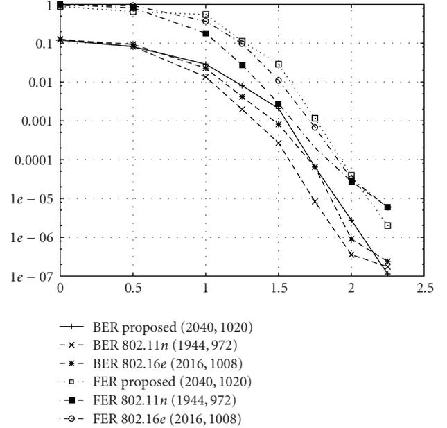
FIGURE 5: Simulation results for code rate 1/2.
