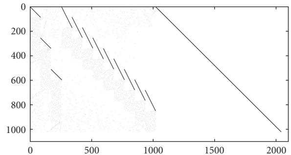
FIGURE 2: Parity-check matrix of a (2040, 1020) code.
