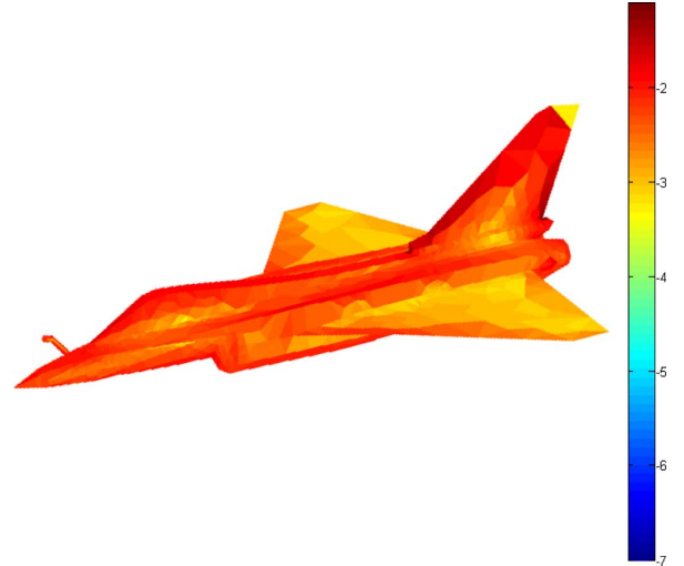
Fig. 18. Aircraft: absolute value of the current (dB).
