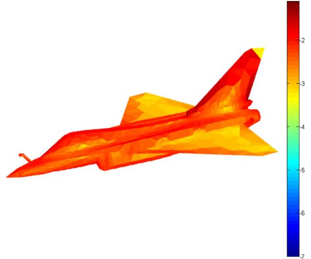
Fig. 18. Aircraft: absolute value of the current (dB).
