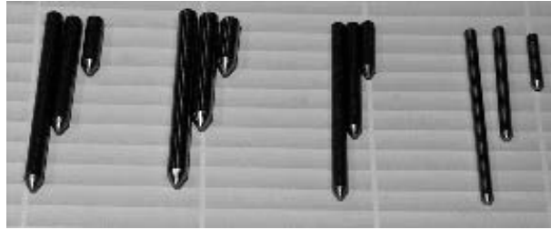
Figure 5: Steel cylinders employed for runners imprinting.
