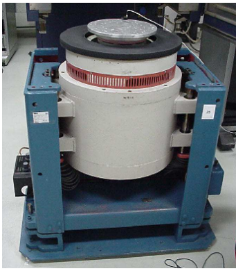
Figure 3. Example of a shaker for CD player test.
