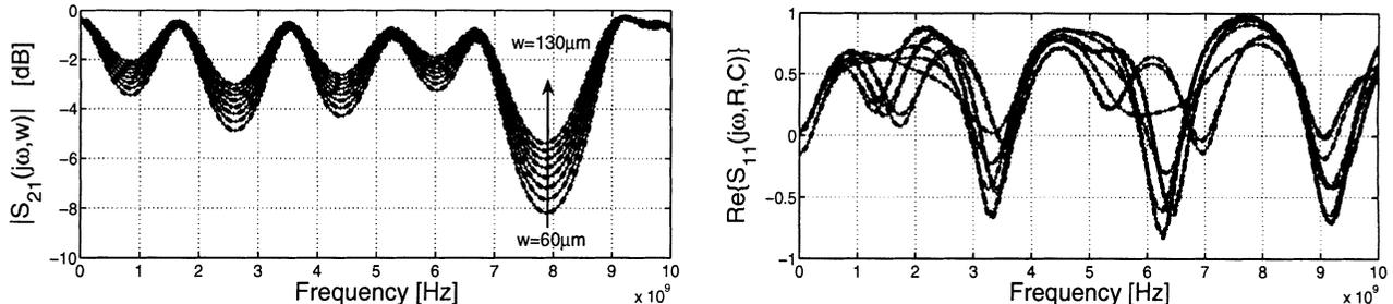
Figure 2: Left: Magnitude of the  $S_{21}$  response of the test circuit (solid line) and of the macromodel (dash-dot line) for different values of the microstrip width  $w$ . Right: Real part of the  $S_{11}$  coefficient of the true system (solid line) and of the model (dash-dot line) for different values of  $R$  and  $C$  (for clarity, only some validation responses are shown).
