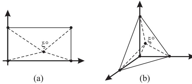
Figure 1: A domain of size  $\sigma$  is broken into  $\sigma$  sub-domains by joining the point  $\xi^\circ = (\xi_1^\circ, \xi_2^\circ, \dots, \xi_\sigma^\circ)$  to each domain vertex. The figure illustrates the case for elements of size four: a) the two-dimensional quadrilateral element is subdivided about the point  $\xi^\circ$  into four triangular sub-domains; b) the three-dimensional tetrahedral element is broken about the point  $\xi^\circ$  into four tetrahedral sub-domains.
