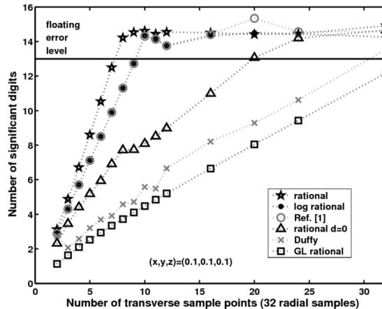
Figure 4: Convergence comparison for a nearly singular integral over  $T$ , with observation point  $(x, y, z) = (0.01\lambda, 0.01\lambda, 0.01\lambda)$ , and  $\Lambda(\mathbf{r}) = 1$ . In the body of the figure the global coordinates of the observation point are reported in meters.
