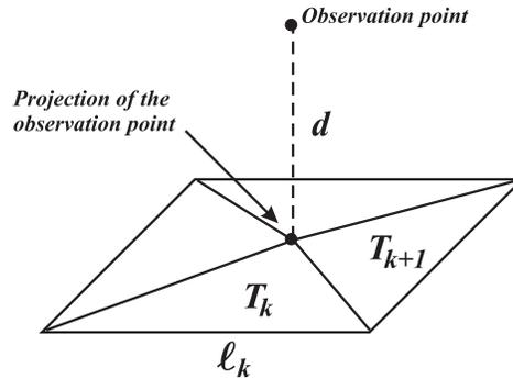
Figure 2: A four-sided planar patch of the object space is broken into four triangular subdomains about the normal projection  $\mathbf{r}_p$  of the observation point  $\mathbf{r}$  onto the plane of the patch; the distance from  $\mathbf{r}$  to the plane of the patch is  $d$ .
