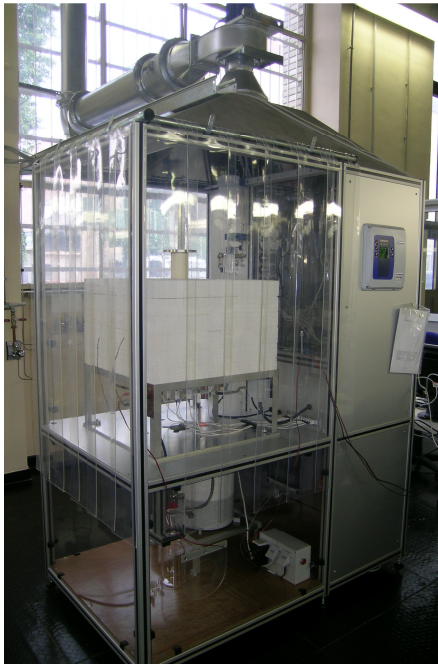
Figure 2. Experimental setup for the testing of planar cells
