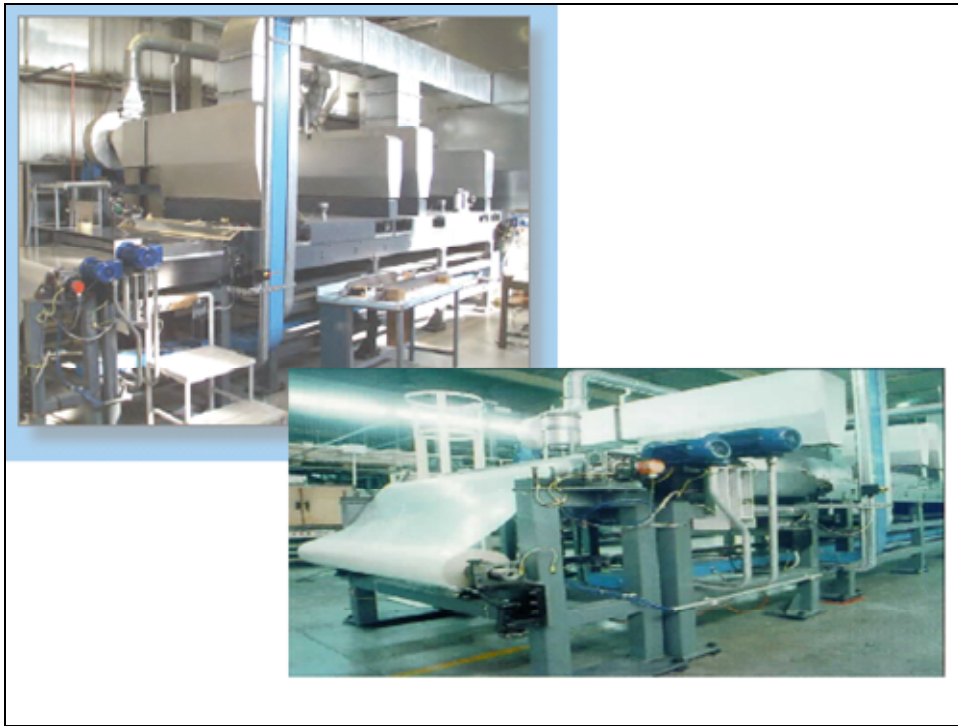
Figure 1. Industrial tape-caster machine for preparation of SOFC anode supports installed at FN Nuove Tecnologie e Sistemi Avanzati S.p.A.
