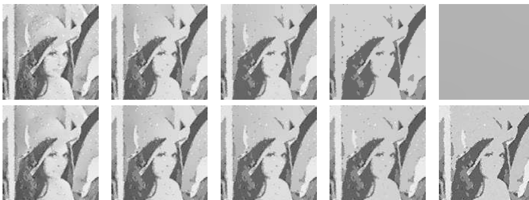
Fig. 3. Top: Perona-Malik model. Bottom: Polynomial CNN. From left to right: Output images at the scales t = 0.1 , t = 1 , t = 10 , t = 100 and t = 500 .
