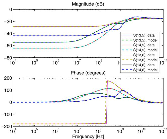
Fig. 9. Comparison between raw scattering data and fitted model for the LNA structure. Couplings between non-inverting inputs at 1800 MHz (port 5) and 1900 MHz (port 6) to power supply ports  $V_{DD}$  (port 13) and  $V_{SS}$  (port 14) are shown.
