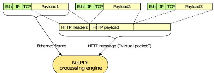
Figure 3. Processing *real* and *virtual* packets in NetPDL.
