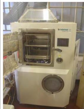
Figure 7. The pilot freeze-dryer used for experiments
