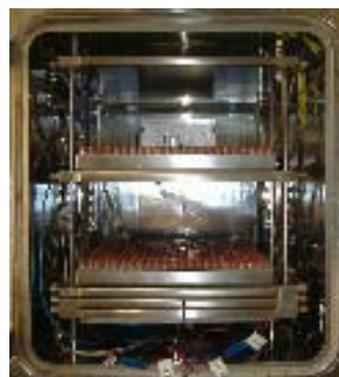
Figure 6. Balance positioned inside the vacuum chamber
