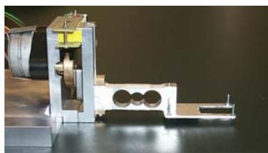
Figure 3. Lifting system.
