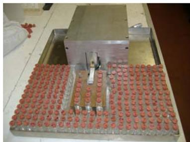
Figure 5. Balance positioned on a tray in a batch of vials.
