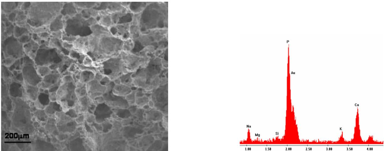
Fig. 4 I-CEL2 scaffold SEM micrograph (a) and EDS analysis of the scaffold surface (b)
