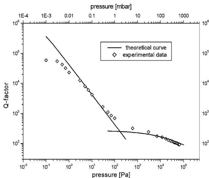
FIG. 4. Experimental evaluation for the quality factor (open diamonds) as a function of the pressure and comparison with the theoretical curve (solid line). The dimensions of the cantilever beam are  $800 \times 100 \times 5 \mu\text{m}^3$ .
