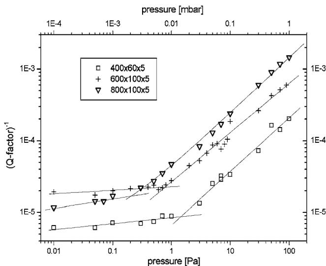
FIG. 6. Comparisons of pressure response for different cantilevers in molecular region. Drawn lines are fit of experimental values. Geometrical dimensions are, as usual, (length)  $\times$  (width)  $\times$  (thickness)  $\mu\text{m}^3$ .
