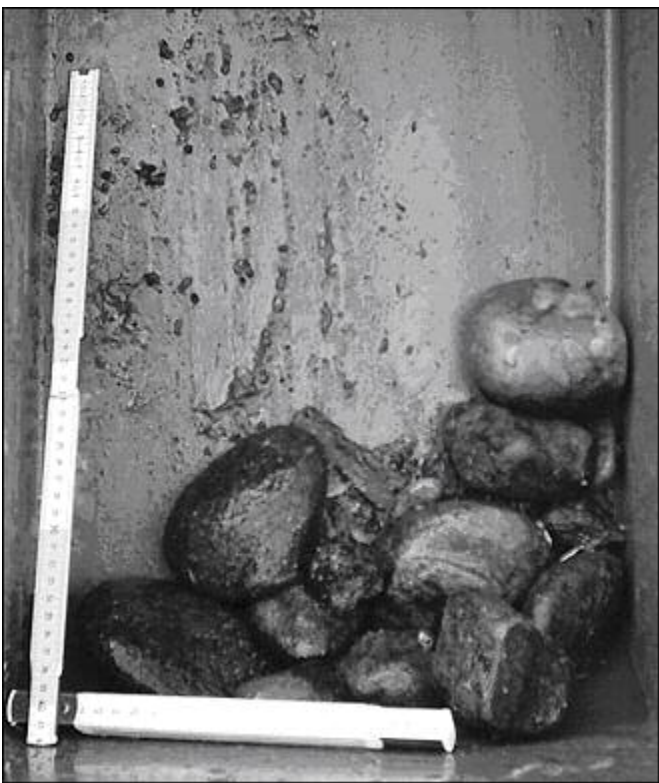
Figure 9 □ Example of coarse riverbed sampled material.
