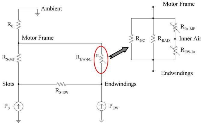
Fig. 9. Proposed simplified thermal model for the prototype.
