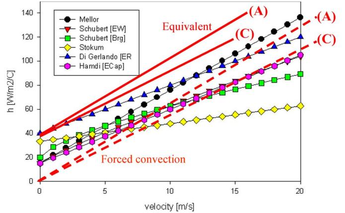
Fig. 17. Comparison between the estimated heat-transfer coefficients with the published ones. (A) MA160 motor prototype; (C) MA112 motor prototype.
