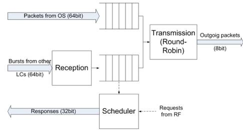
Fig. 5. Outgoing packets management structure
