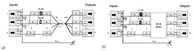
Figure 3. Interconnection architecture a) with amplifiers b) with AWG.
