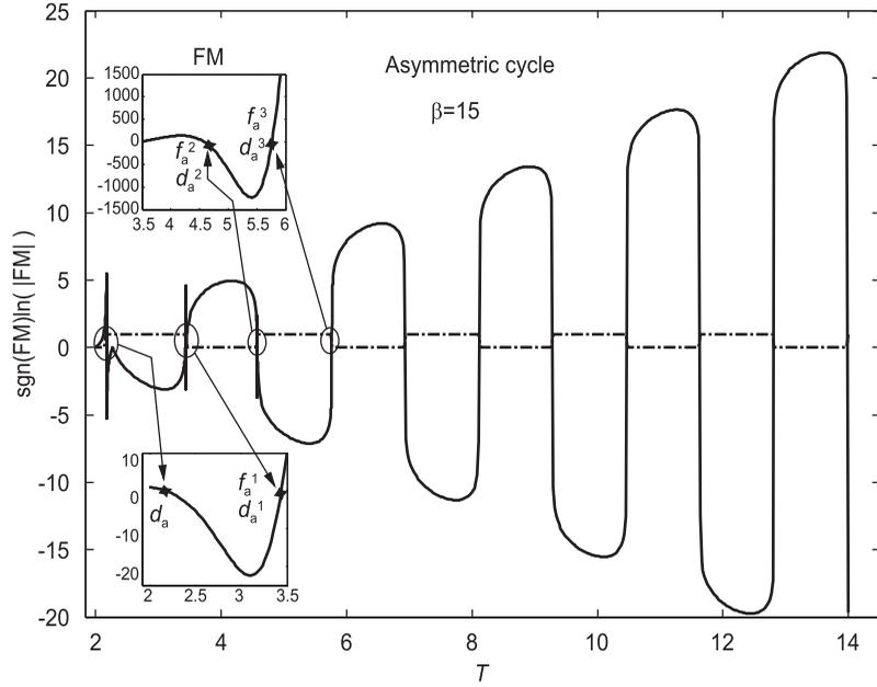
Figure 5. Chua's circuit:  $T$  dependence of the real part of the FM responsible of bifurcations for the asymmetric limit cycle. The dash-dotted line represents a function equal to 0 if the FE nearest to the real axis is real, and to 1 if it is complex.
