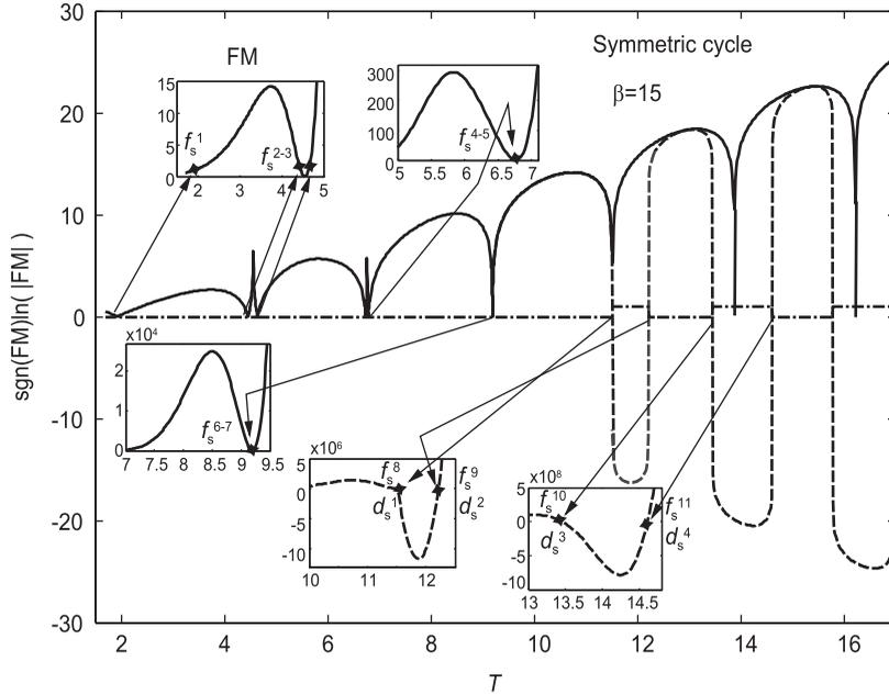
Figure 3. Chua's circuit:  $T$  dependence of the real part of the FM responsible for bifurcations of the symmetric limit cycles. The dash-dotted line represents a function equal to 0 if the FE nearest to the real axis is real, and to 1 if it is complex.
