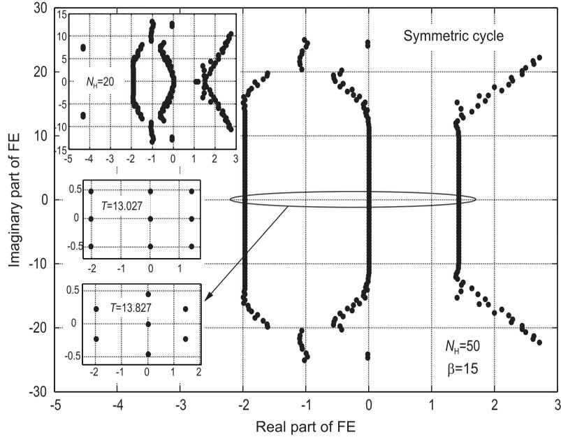
Figure 2. Chua's circuit: example of FE distribution in the complex plane for the symmetric limit cycle ( $N_H = 50$ ,  $T = 13.827$ ). Top inset: FE distribution for  $N_H = 20$ ,  $T = 13.827$ . Middle inset: zoom of the FE distribution for  $T = 13.027$ . Bottom inset: zoom of the FE distribution for  $T = 13.827$ .
