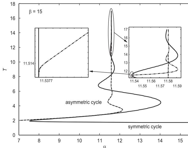
Figure 1. Chua's circuit:  $\alpha$ -parameter dependence of the limit cycle period  $T$  for symmetric and asymmetric cycles. Symmetric cycle: continuous and dash-dotted lines. Asymmetric cycle: dashed line.
