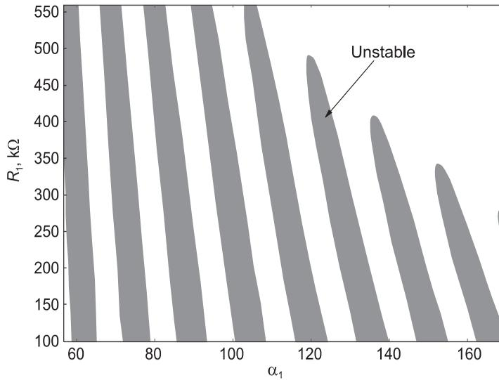
Figure 10. Colpitts oscillator: regions of unstable operation in the  $(\alpha_1, R_1)$  parameter plane. The frontiers of the shaded regions represent fold bifurcation curves, since the FM is real and positive.
