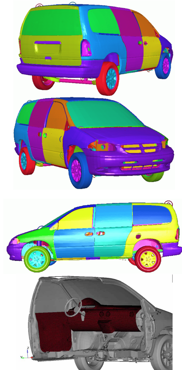
Figure 3. The GCM4 exterior and, below, a view of the interior parts (seats are not shown but are included in the model).
