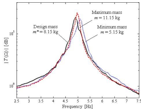
Figure 11: Experimental transmissibility of the elasto-magnetic suspension
