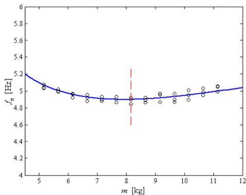
Figure 10: Natural frequency vs. mass for the elasto-magnetic suspension (circles refer to experimental data)
