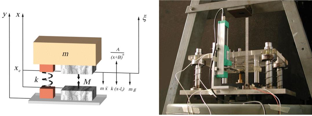
Figure 1: Model (left) and experimental set-up (right) of the elasto-magnetic suspension
