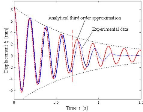
Figure 7: System free response for the elasto-magnetic suspension
