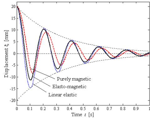
Figure 3: System free response from non-zero initial conditions
