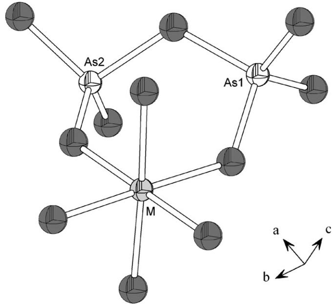
Fig. 2. Perspective view of  $M\text{As}_2\text{O}_{11}$  unit,  $M = \text{Fe}_{0.22}\text{Al}_{0.78}$ .
