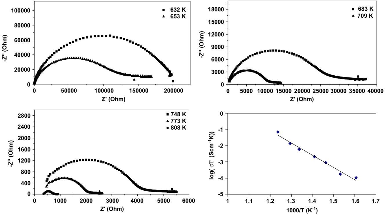
Fig. 4. Complex impedance diagrams  $-Z''$  vs.  $Z'$  for  $\text{TlFe}_{0.22}\text{Al}_{0.78}\text{As}_2\text{O}_7$  over the temperatures ranges 623–653, 683–709 and 748–808 K and Conductivity plot  $\log(\sigma T) = f(10^3/T)$ .
