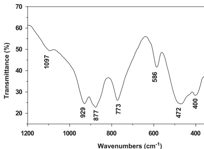
Fig. 3. Infrared analysis spectrum of  $TlFe_{0.22}Al_{0.78}As_2O_7$ .
