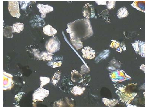
Photo 2. 100 - 200 mesh class. A thin chrysotile tuft at the centre. Short side of the photogram 0,94 mm.
