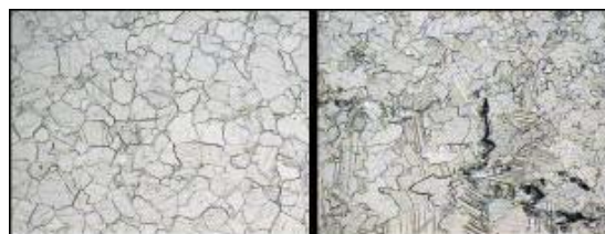
Fig. 2: Microphoto of a granoblastic marble (on the left) and a xenoblastic marble (on the right). Real dimensions 1,9x2,5 mm.
