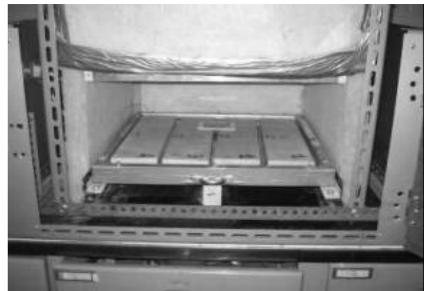
Fig. 12: Apparatus for the execution of the Lab Bow test.
