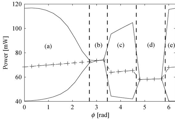
Fig. 7. Maximum, average and minimum output power as functions of the total phase variation. In (a), (c) and (e), the laser is SP; in (b) and (d), it is monomode.
