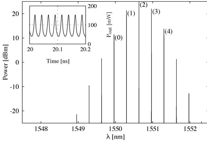
Fig. 4. Same as Fig. 3, but with  $I_a = 300$  mA (region (E) in Fig. 2). SP frequency of 41.74 GHz. The spectral power distribution is in good agreement with the experimental results in [9].
