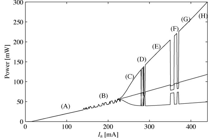
Fig. 2.  $P - I_a$  curve of the SP-3S DBR when  $\alpha_H = 4$  and for the parameters in Table I. The three curves indicate the maximum, the mean and the minimum output power. (A) CW operating region. (B) CW bistable region. (C), (E), (G) SP regions. (D), (F) Transition between different SP behavior. (H) Irregular behavior.
