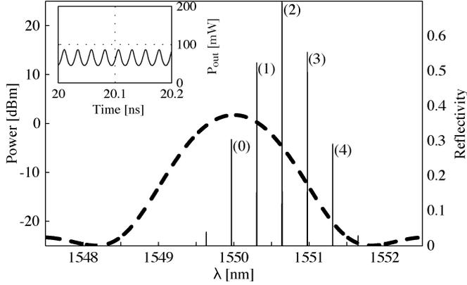
Fig. 3. Optical spectrum for the laser in the first SP region (region (C), Fig. 2). Grating power reflectivity with  $\lambda_B = 1550$  nm: dashed line. In the insert: instantaneous output power. SP frequency of 41.58 GHz.
