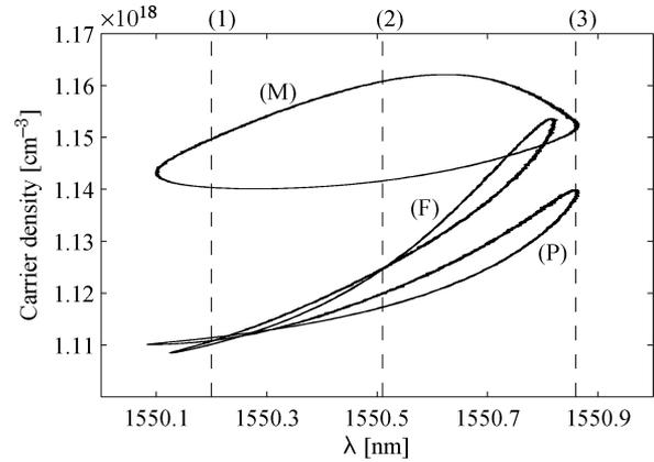
Fig. 12. Periodic pulsations in the carrier density–instantaneous wavelength plane when  $\alpha_H = 4$  and  $I_a = 300$  mA. The three trajectories are calculated using the carrier density in the middle of the active region (M), near the phase control section (P), and near the cleaved facet (F). The dashed lines indicate the position of modes 1–3 of Fig. 4.
