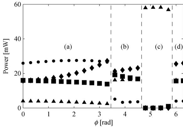
Fig. 10. Mode output power as in Fig. 8 when  $\alpha_H = 6$  and  $I_a = 269$  mA ( $\blacktriangle$ : mode 0,  $\blacksquare$ : mode 1,  $\blacklozenge$ : mode 2,  $\bullet$ : mode 3). In regions (a), (b), and (d), the device is SP, while in (c) it is monomode.
