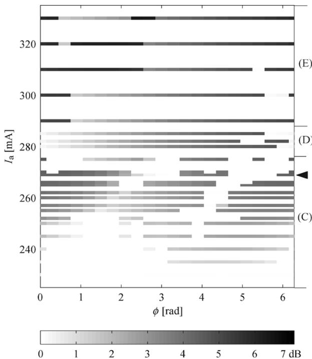
Fig. 11. Ratio between the maximum and the minimum values extracted from the temporal evolution of the output power (in decibels) when  $\alpha_H = 4$ , for different values of  $I_a$  and  $\phi$ . The dark segments on the horizontal bars correspond to better SP conditions, whereas the white bars to CW behavior. Regions (C), (D), and (E) refer to Fig. 2. The arrow ( $\blacktriangleleft$ ) indicates the case with  $I_a = 269$  mA presented in Fig. 7.
