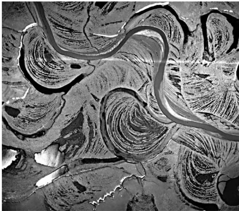
Figure 1. An aerial photograph of the Colville River (Alaska). Enlargement and continuous migration of meanders as well as the formation of cutoffs can be observed.
