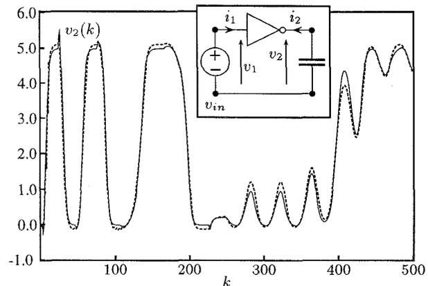
Figure 5: Waveform  $v_2(k)$  of the circuit of the insert for a validation input  $v_{in}$ . Solid curve: reference response; dashed curve: response produced by the NARX MIMO inverter model described in the text
