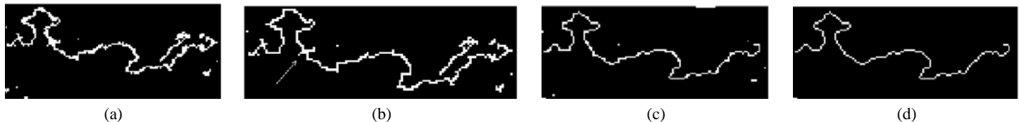
Fig. 3. Example of some image processing steps, zoom on one molecule in an AFM image: (a) molecule after thresholding; (b) molecule after thinning. The arrow in the image (b) shows one of the spurious branches; (c) same molecule after pruning and Critical molecules removing: the isolated fragment on the right in (a) and (b) has been removed in (c); (d) same molecule at the end of the processing
