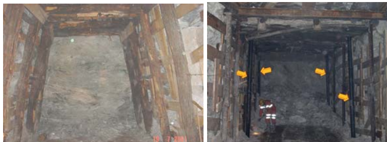
Figure 1. View of a drift supported by timber sets and hydraulic (arrows) and mechanical props
