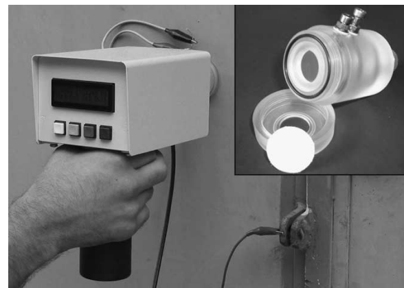
Fig. 2. System during an outside measurement of a common painted metallic door and a detailed photo of the electrochemical cell.
