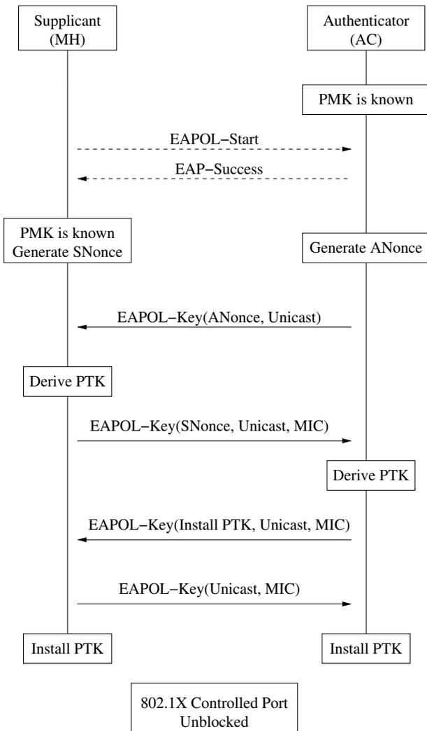
**Figure 3** – Fast Authentication with Four Way Handshake (FWH)
