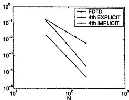
Figure 3: Comparison between FDTD and fourth-order schemes with RK4 time stepping applied to a unmatched scalar transmission line. The plot reports the  $L^\infty$  error on the termination voltage at the right boundary.
