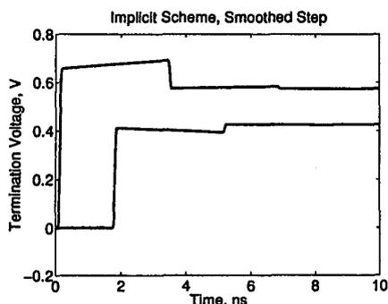
Figure 5: Termination voltages for a high-loss PCB line.
