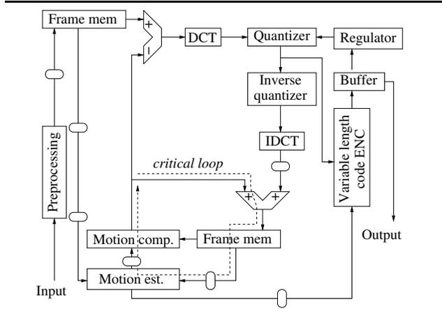
Figure 6. MPEG block diagram with pipelining memory elements.
