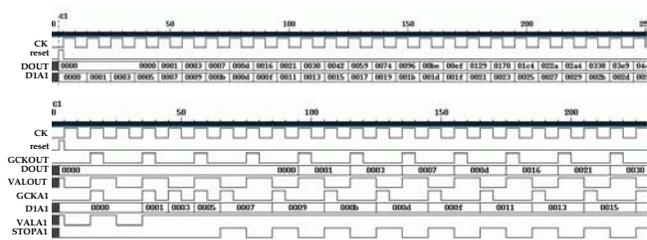
**Figure 4. Snapshots of Simulations for system of figure 3.**
