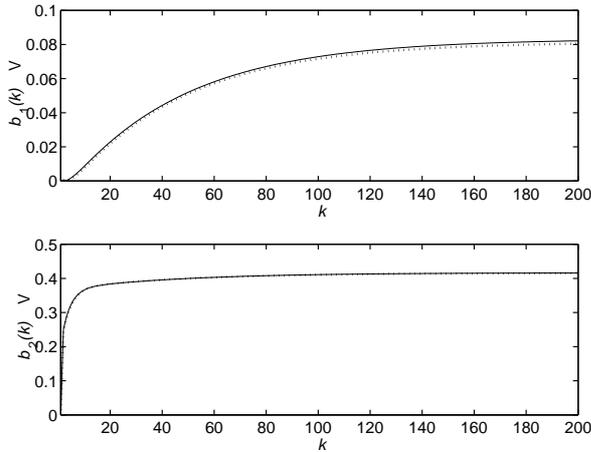
Figure 4: Discrete-time response  $\mathbf{y}(k)$  of the original system and of the estimated model to the input sequence  $\mathbf{u}(k) = [0, 0]^T$ ,  $k < 0$ ;  $\mathbf{u}(k) = [0, 0.5]^T$ ,  $k > 0$ . Solid line: reference response; dotted line: estimated model response.
