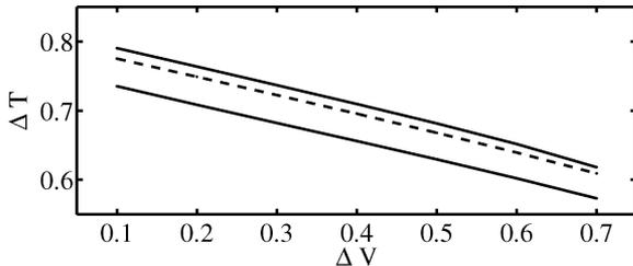
Fig. 8. Eye opening parameter values (defined in Fig. 4) for the eye diagrams of waveforms  $v_2$  computed in test case #2. Solid thin line: reference; solid thick line: macromodels (M1 set); dashed thick line: macromodels (M2 set).
