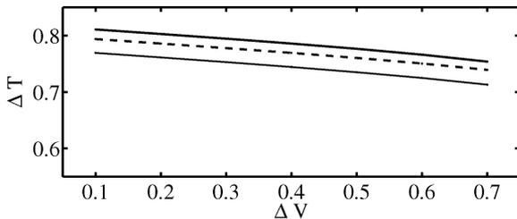
Fig. 9. Eye opening parameter values (defined in Fig. 4) for the eye diagrams of waveforms  $v_3$  computed in test case #2. Solid thin line: reference; solid thick line: macromodels (M1 set); dashed thick line: macromodels (M2 set).
