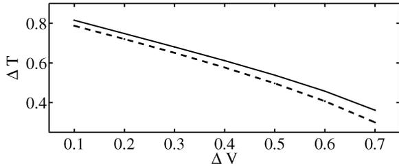
Fig. 13. Eye opening parameter values (like those defined in Fig. 4) for the eye diagrams of waveforms  $v_3$  computed in test case #3 (see Fig. 11). Solid thin line: reference; dashed thick line: macromodels.
