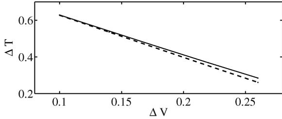
Fig. 12. Eye opening parameter values (defined in Fig. 4) for the eye diagrams of waveforms  $v_{12} - v_{22}(t)$  computed in test case #3 (see Fig. 11). Solid thin line: reference; dashed thick line: macromodels.
