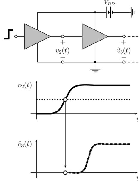
Fig. 2. Ideal setup for recording the basic up state transition of  $\hat{v}_3(t)$  (the dashed-black curve in figure) that is triggered by a suitable voltage crossing of receiver input voltage  $v_2(t)$ .
