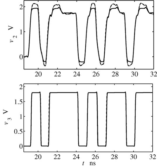
Fig. 3. Voltage waveform  $v_2(t)$  for the test case #1. Solid thin line: reference; solid thick line: macromodels (**M1** set); dashed thick line: macromodels (**M2** set).
