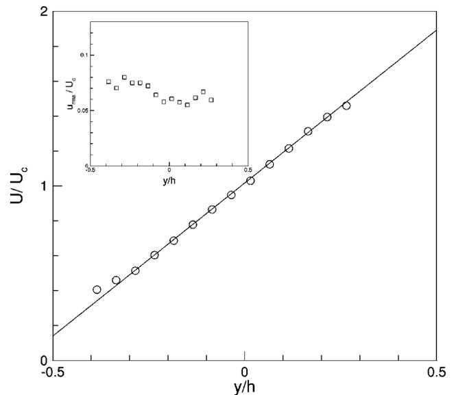
FIG. 1. Homogeneous shear flow: Mean velocity profile as a function of the nondimensional coordinate in the mean gradient direction,  $y/h$ . In the inset, the normalized streamwise turbulent intensity  $u_{rms}$ . Velocities are normalized in terms of the centerline velocity,  $U_c=10.2 \text{ m s}^{-1}$ , while the test section height is  $h=0.9 \text{ m}$ .
