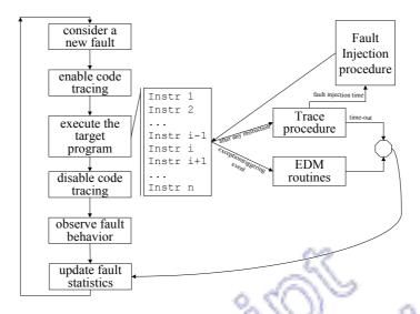
Figure 2: Fault Injection Manager operation flow.
