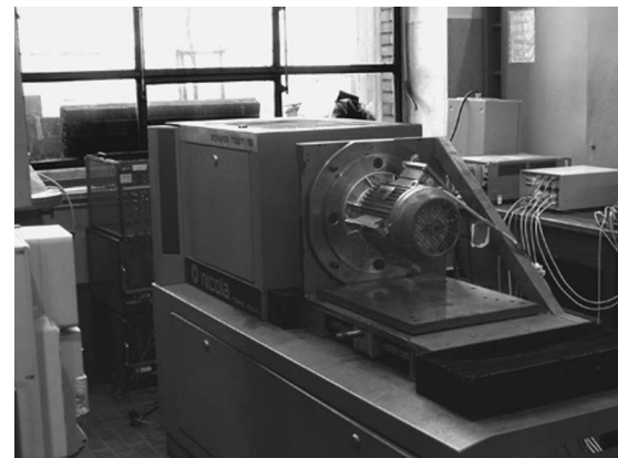
Fig. 4. Test bench for the ac load test.
