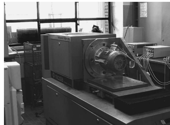
Fig. 4. Test bench for the ac load test.
