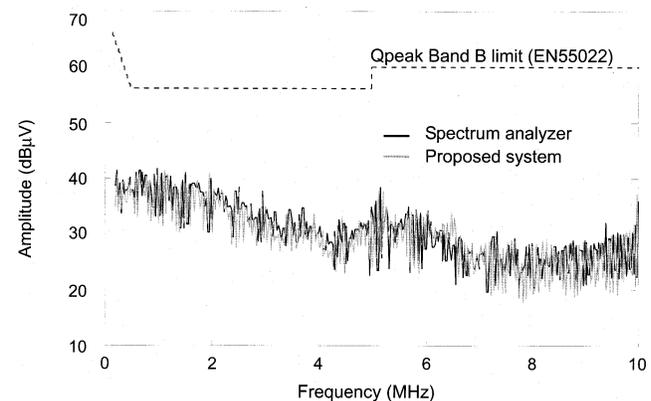
Fig. 4. Conducted emissions of a personal computer.
