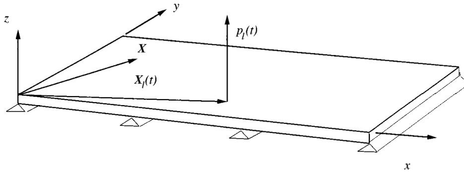
Figure 1. Continuous model of the bridge.
