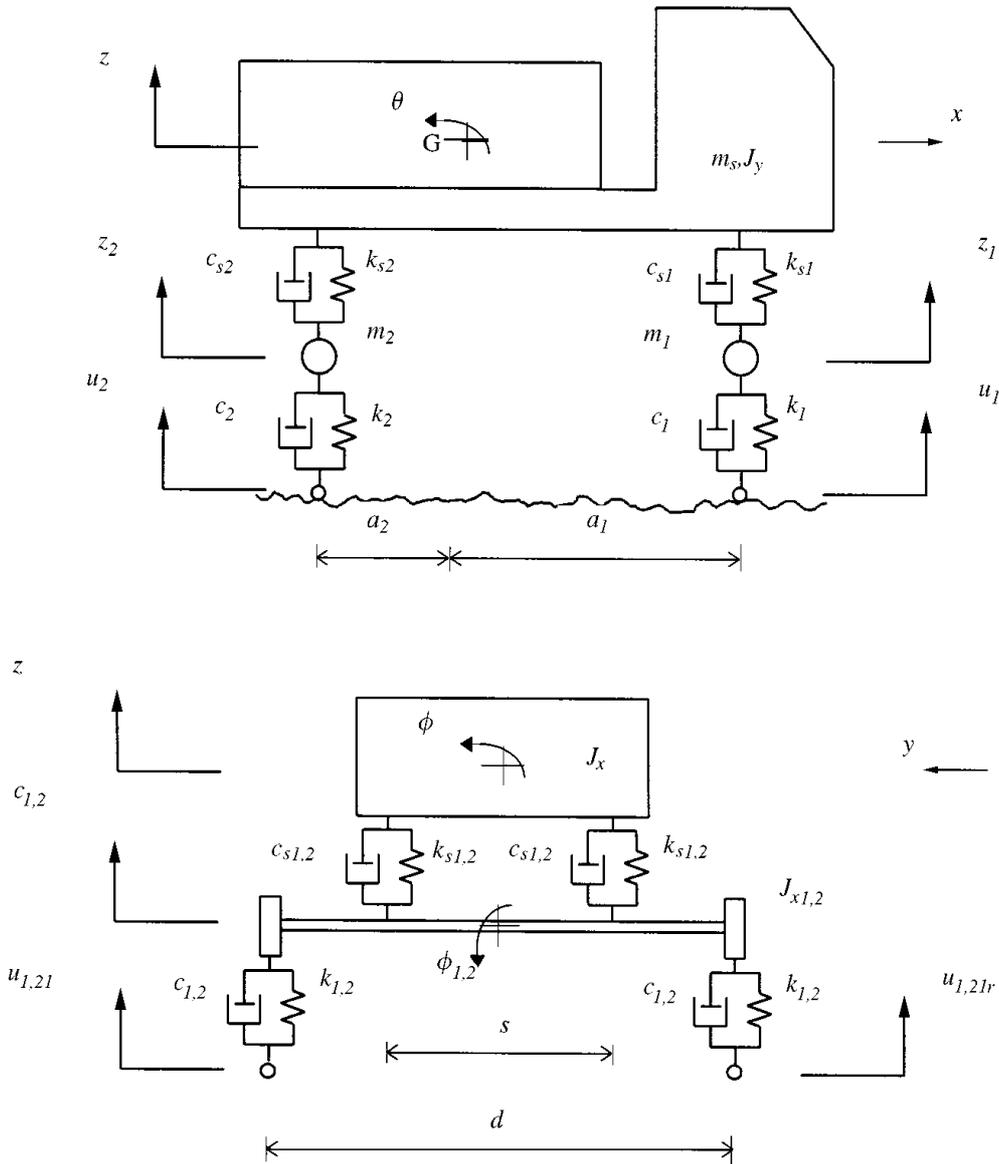
Figure 3. Sketch of the seven d.o.f. system and its parameters.  $z, z_1, z_2$  = vertical displacement of body, front and rear axle;  $\theta$  = pitch displacement of the body;  $\phi$  = roll displacement of the body;  $\phi_1, \phi_2$  = front and rear axle angular displacements;  $u_{1b}, u_{1r}, u_{2l}, u_{2r}$  = road displacements under left front, right front, left rear, right rear tyre.
