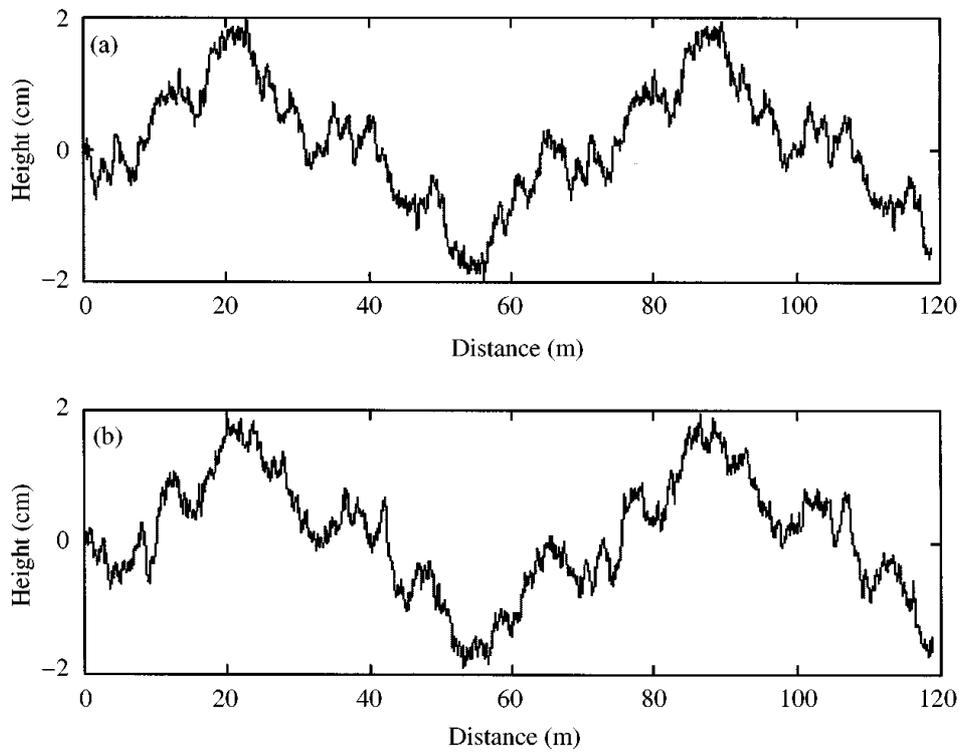
Figure 13. Vertical surface profiles of a damaged road: (a) left line; (b) right line. The lower and upper cut-off spatial frequencies are  $\gamma_0 = 0.015$  cycles/m and  $\gamma_J = 10$  cycles/m, respectively.
