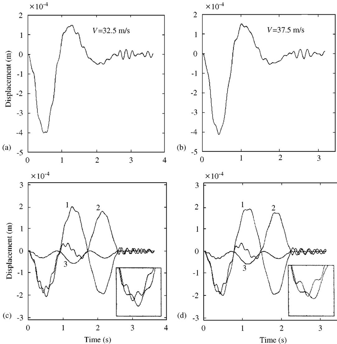
Figure 11. Time histories relative to deflections in point 2 for two different speeds. (a) and (c) correspond to the point marked by “O” in Figure 8; (b) and (d) correspond to the point marked by “+” in the same figure. In figure (c) and (d) the mode contributions are highlighted.
