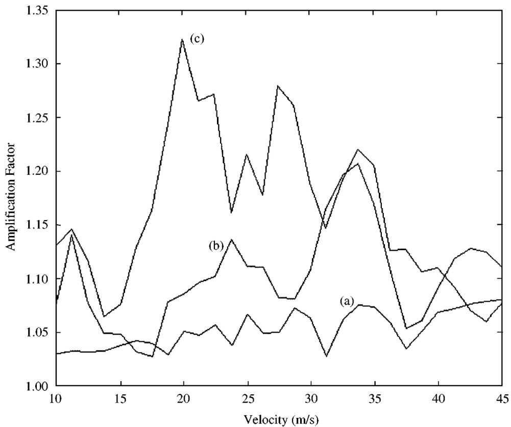
Figure 15. Amplification Factor relative to point 5 versus vehicle speed for a smooth (a) and rough (b) surface (Figure 13). The curve (c) refers to a rough surface and to very small values of suspension damping (the damping matrix of the vehicle-system is reduced to one-tenth of the original).
