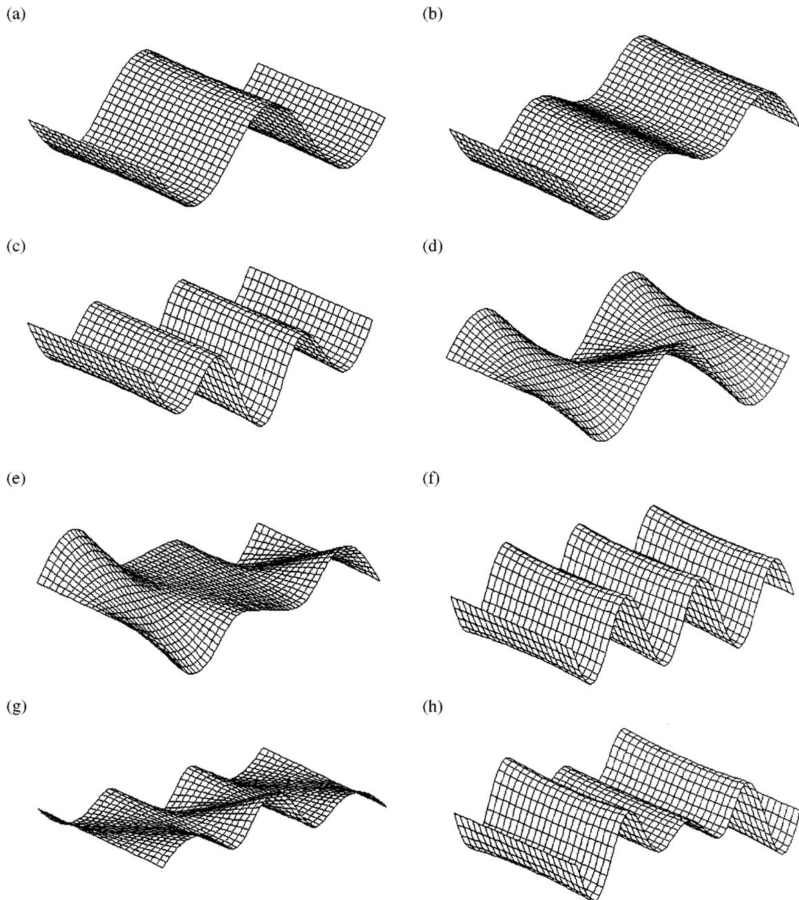
Figure 7. First eight modes of the bridge. Modes: (a) 1,  $f = 4.79$  Hz; (b) 2,  $f = 6.19$  Hz; (c) 3,  $f = 9.11$  Hz; (d) 4,  $f = 16.65$  Hz; (e) 5,  $f = 17.55$  Hz; (f) 6,  $f = 19.37$  Hz; (g) 7,  $f = 19.57$  Hz; (h) 8,  $f = 22.16$  Hz.
