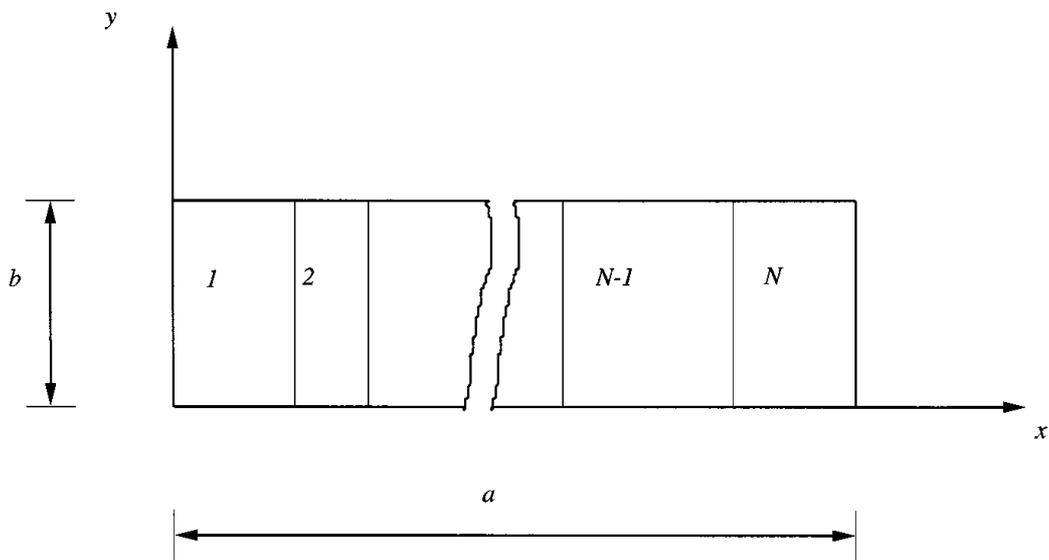
Figure 2. *N*-span continuous rectangular plate.
