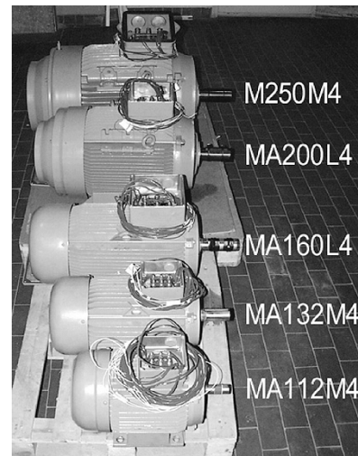
Fig. 1. TEFC motors used to generate test data.
