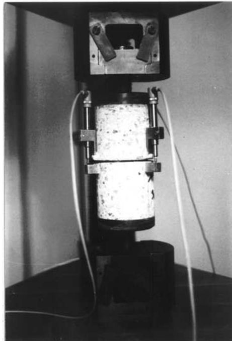
Figure 2: Tensile test setup.
