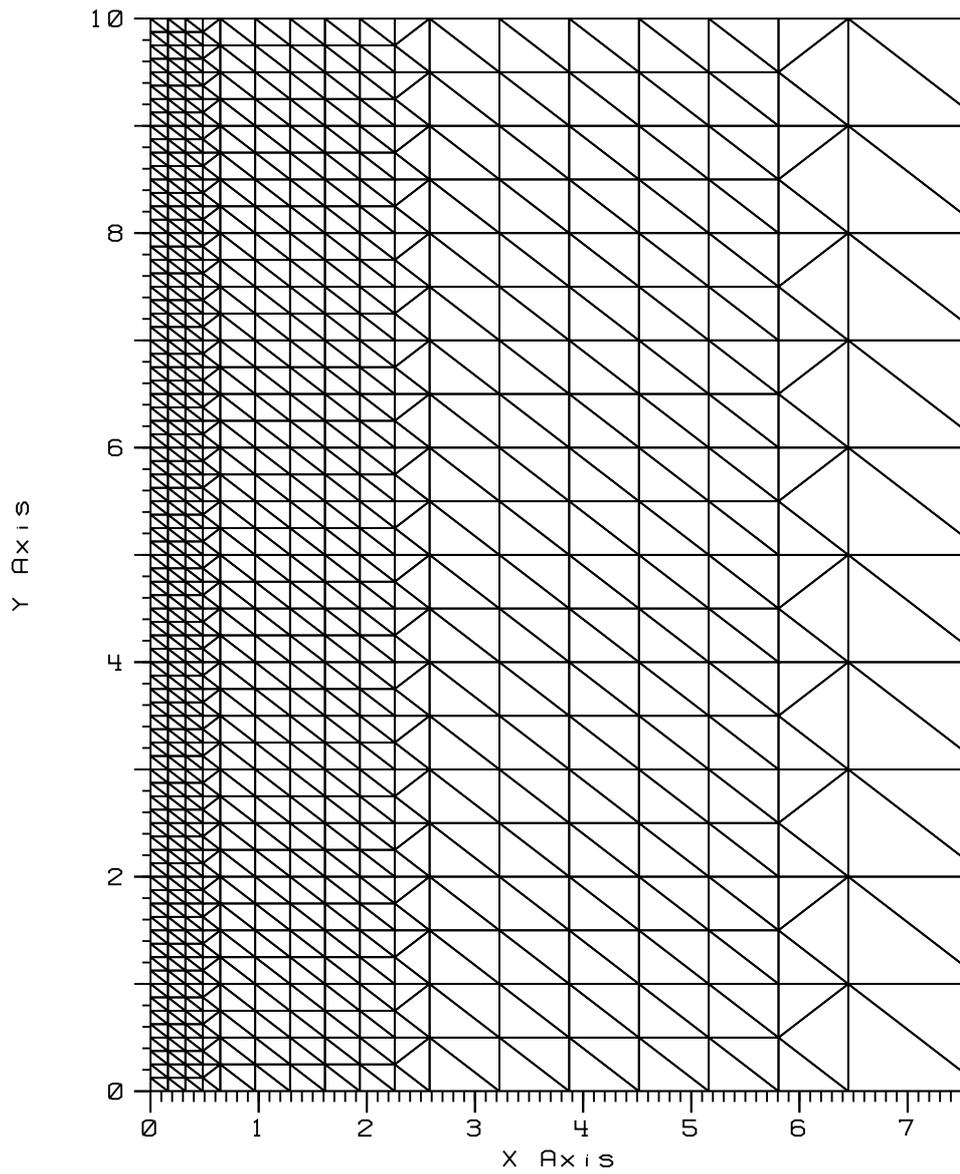
Figure 6: Portion of the finite element mesh around the symmetry axis (dimensions in centimeters).
