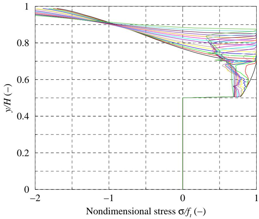
Figure 9: Stress distribution inside the process zone.
