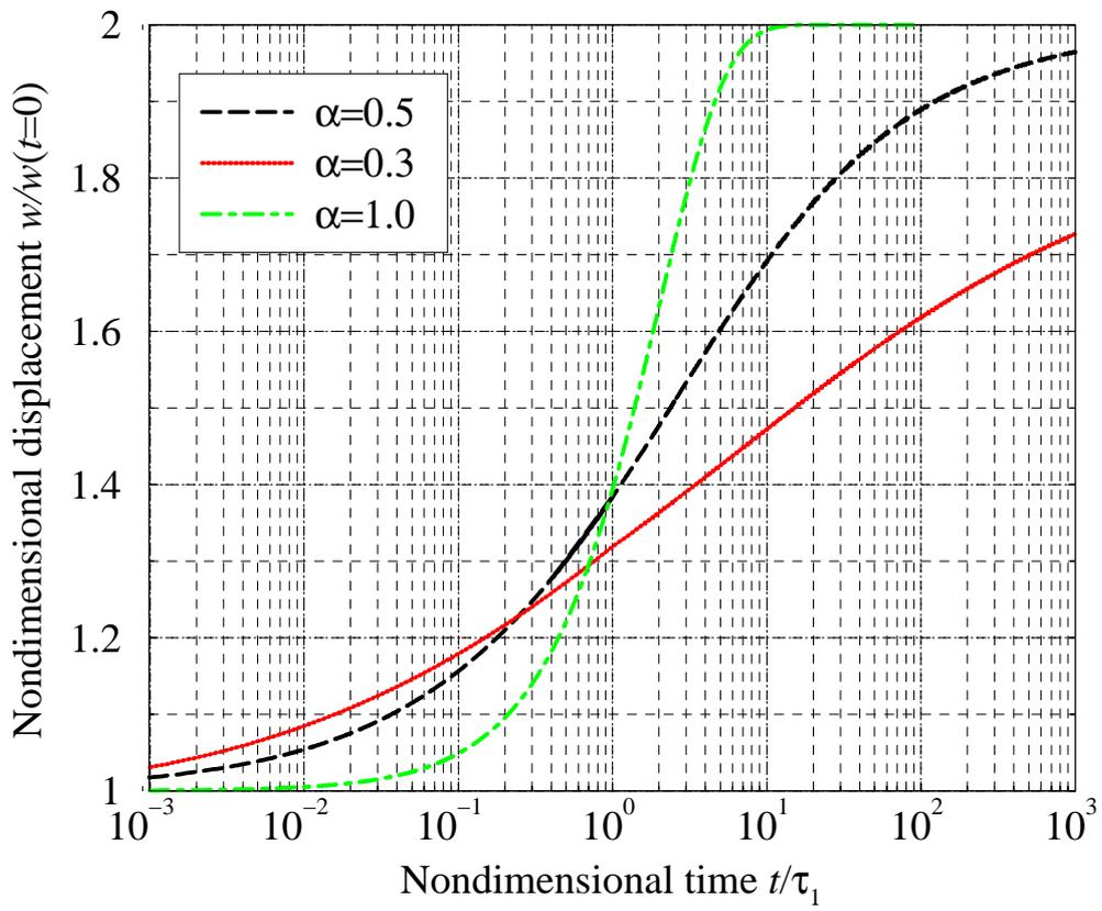
Figure 3: Creep displacement functions ( $E_1 = E_2$ ).
