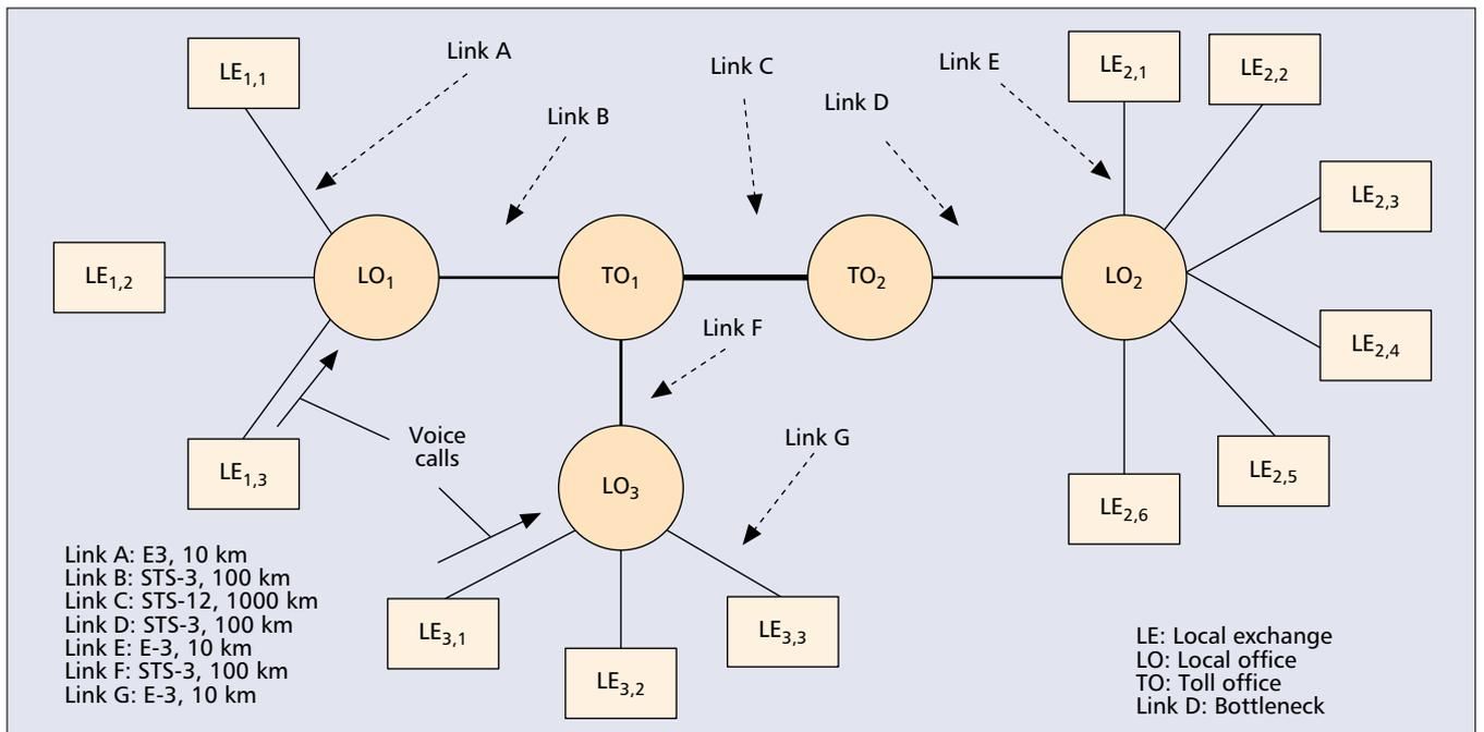
■ **Figure 1.** The network topology used in simulations.
