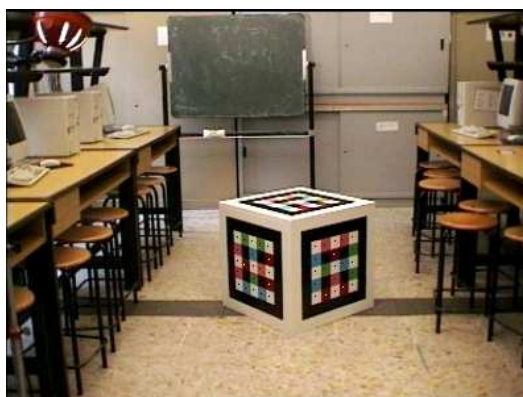
Figure 68: reference points on a calibration object, and their position on the image plane
