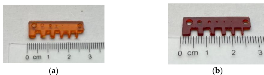
Figure 7. Definition printing object of E1 (a) and D1 (b) resin.
