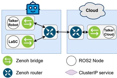
Fig. 1: Architecture interconnecting cloud and robot cluster.
