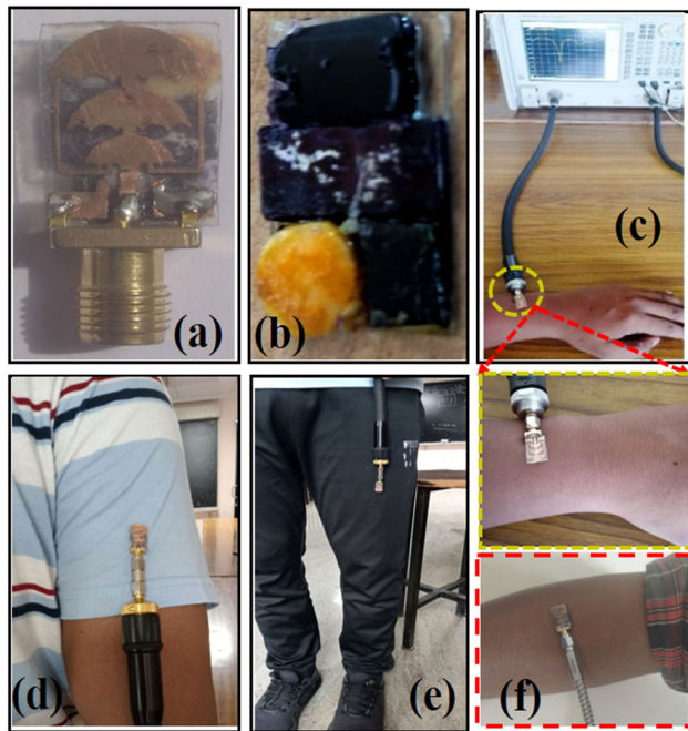
FIGURE 13. Experimental setup (a) Fabricated prototype with integrated circuit, (b) assembled electronic circuitry (c) near-field measurement setup for on-wrist scenario, (d) on-bicep scenario and, (e) on-thigh scenario, (f) on-forearm for validation of flexible characteristics.
